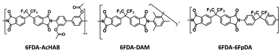
Fig. 3 Chemical structure of the monomers and selected final polyimides.
