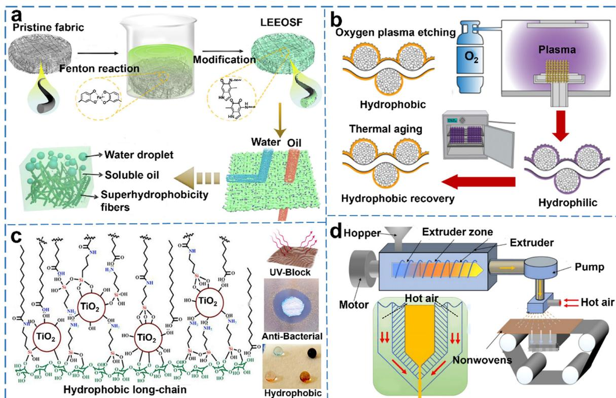
Fig. 4 Preparation of superhydrophobic fabric by (a) Fenton reaction,<sup>116</sup> Copyright 2023 Elsevier; (b) oxygen plasma etching and thermal aging,<sup>117</sup> Copyright 2020 Elsevier; (c) hydrophobic branches on fabric long chains,<sup>118</sup> Copyright 2023 Elsevier; (d) melt-blow method,<sup>119</sup> Copyright 2022 MDPI.
