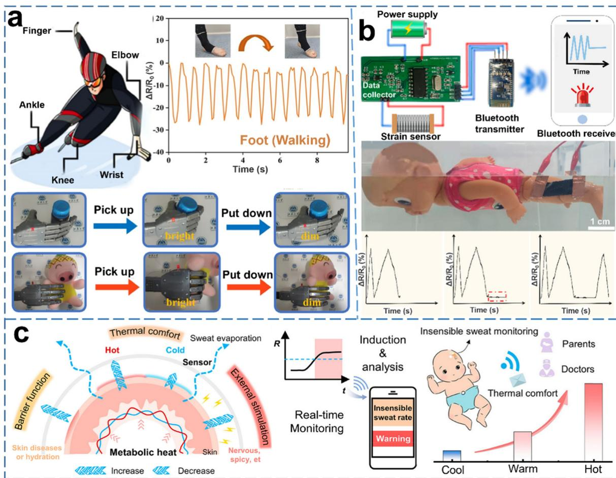
Fig. 12 (a) Multifunctional fabric sensor,<sup>200</sup> Copyright 2022 Springer Nature; (b) drowning alarm device based on fabric,<sup>202</sup> Copyright 2022 American Chemical Society; (c) application of conductive fabric in medical treatment,<sup>201</sup> Copyright 2023 American Chemical Society.
