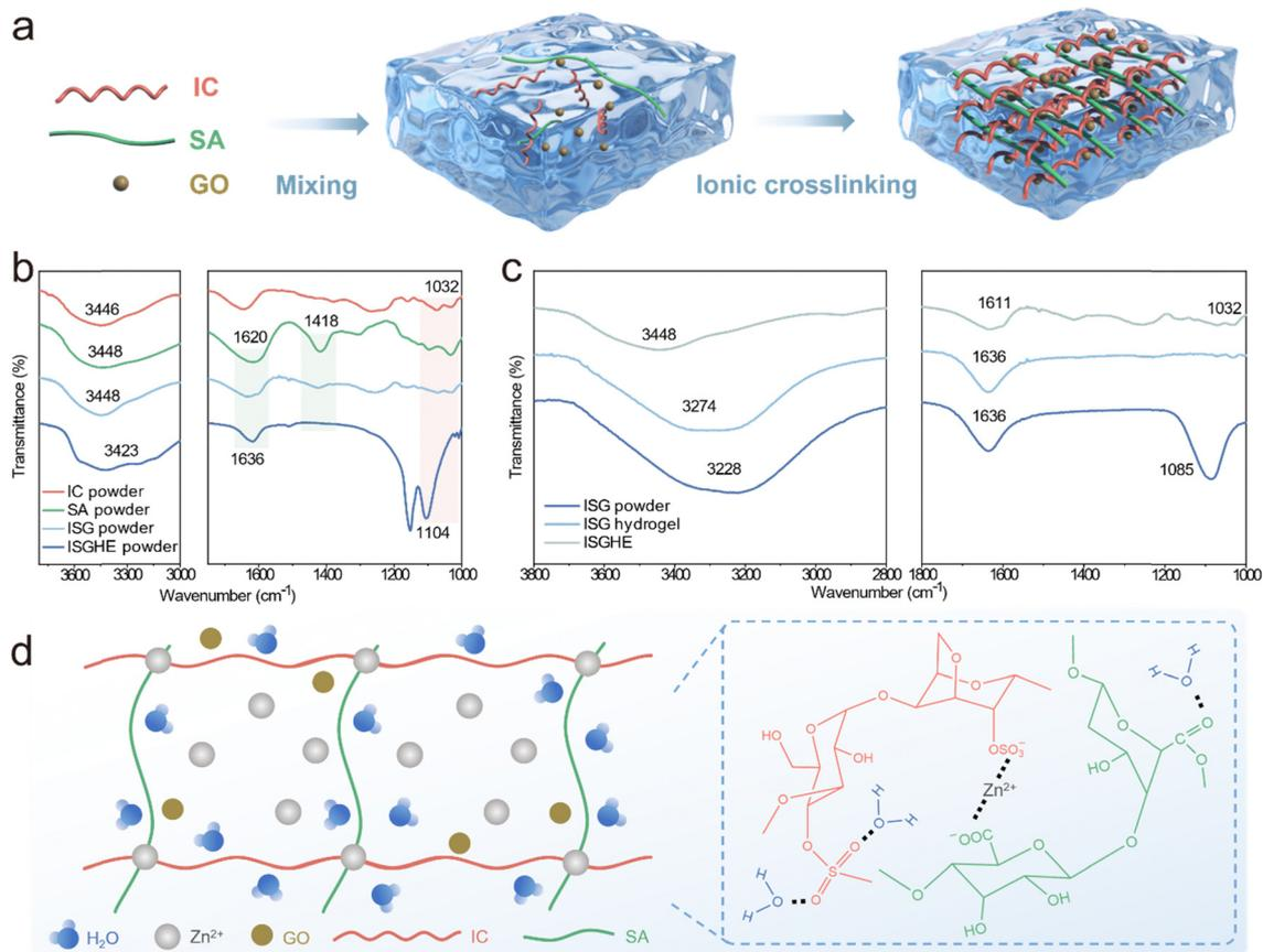
**Fig. 1** Fabrication and characterization of the ISGHE. (a) Schematic illustration of the fabrication process of the ISGHE. (b) FTIR spectra of ISG, SA, ISG and ISGHE powders in the dry state. (c) FTIR spectra of the ISG powder, ISG hydrogel and ISGHE. (d) Schematic illustrations of the cross-linking mechanisms.
