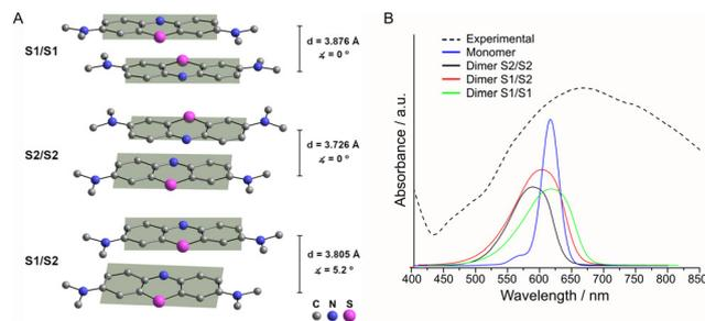
Fig. 6 (A) Representation of the dimers in the MB columns. (B) Diffuse reflectance spectrum of **MBV<sub>10</sub>** (dashed) and calculated absorption spectra for the MB monomer and for the dimers at the X3LYP/Def2-TZVP/SMD theory level.
