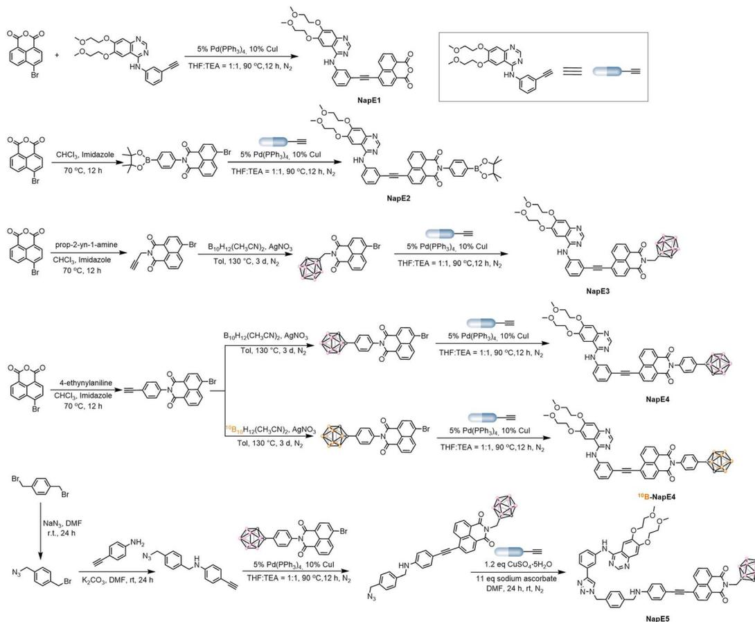
Fig. 2 Synthesis of five carborane-based boron delivery agents.
