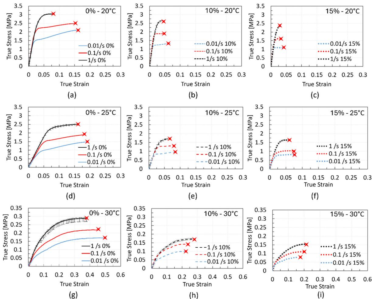
Fig. 4  $\sigma$ - $\epsilon$  data for chocolate samples of different porosities from the uniaxial compression tests under three strain rates at 20 °C, 25 °C, and 30 °C. The red "x" marks indicate the location where ultimate failure occurs.
