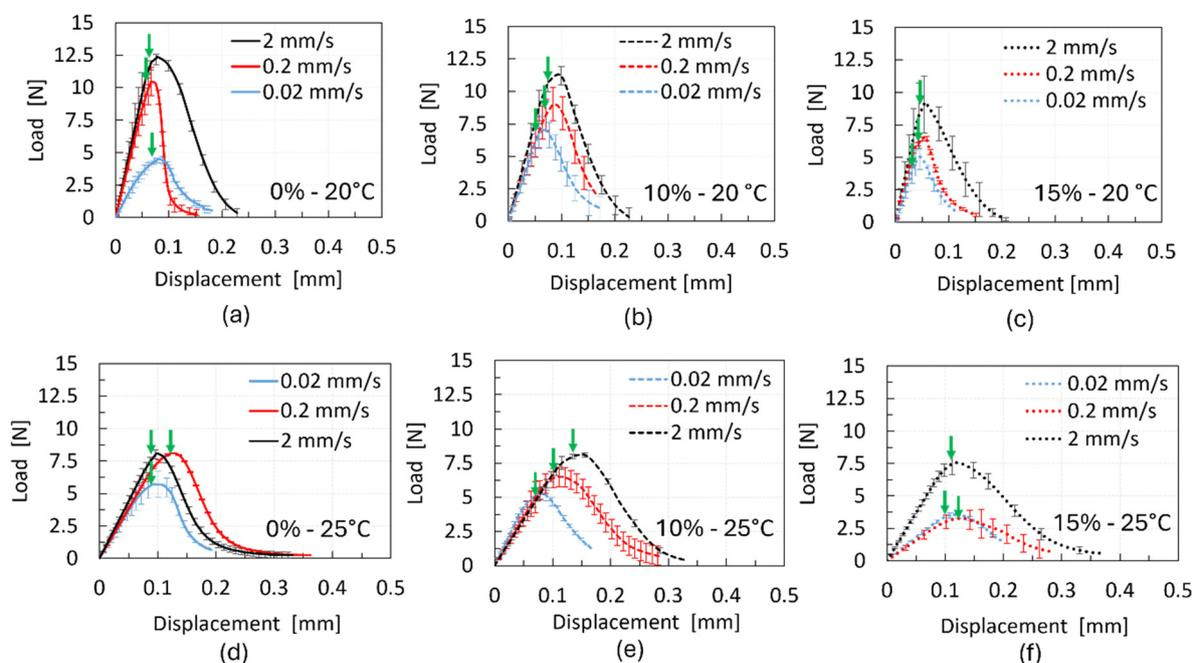
**Fig. 8** Load-displacement data for chocolate materials of different porosities from the SENB tests under three testing speeds at  $20^\circ\text{C}$  and  $25^\circ\text{C}$ .
