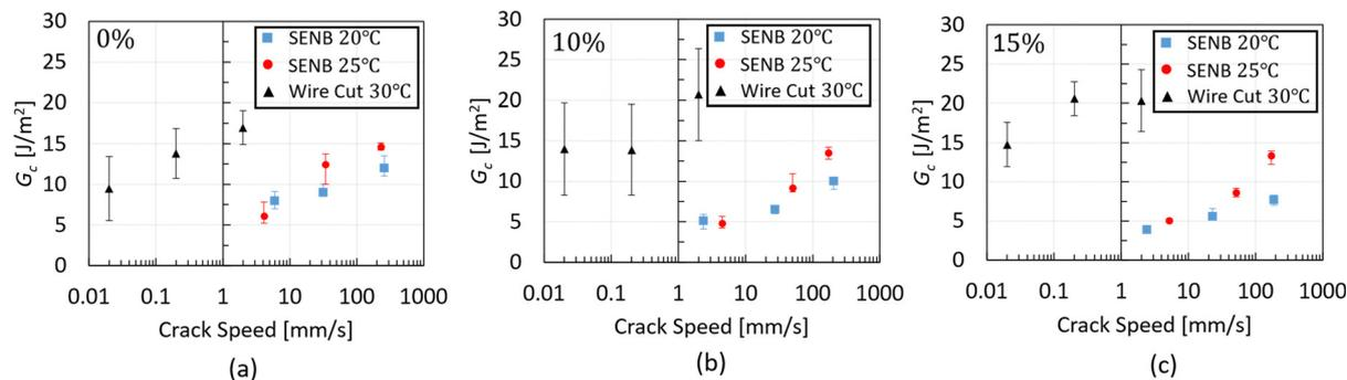
Fig. 13 Graphs summarising  $G_c$  obtained from SENB and wire cutting tests at different temperatures, 20 °C, 25 °C, and 30 °C, as a function of crack speed. Plots show the average values of  $G_c$  of the (a) non-aerated chocolate (0%), (b) 10%, and (c) 15% micro-aerated chocolate.
