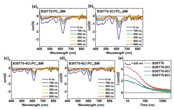
Fig. 5 (a-d) TAS of B30T70-XCl: $PC_{71}BM$  films for time decays up to 500 ns and (e) transient absorption kinetics monitored with 620 nm probe wavelength.
