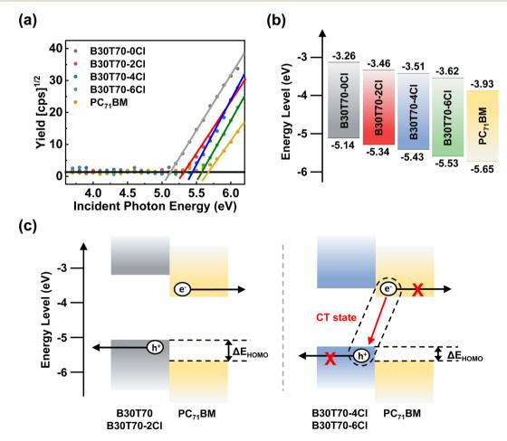
Fig. 3 (a) PESA measurements of B30T70-XCl (X = 0, 2, 4 and 6) and PC<sub>71</sub>BM, along with (b) corresponding energy level diagram. (c) Schematics showing different populations of charge-separated states in B30T70 (or 2Cl) and B30T70-4Cl (or 6Cl) devices.
