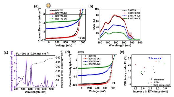
Fig. 2 (a and d) J-V curves of B30T70-XCl (X = 0, 2, 4 and 6):PC<sub>71</sub>BM devices under illumination of 1-Sun and FL 1000 lx, respectively, and (b) corresponding EQE spectra of B30T70-XCl (X = 0, 2, 4 and 6):PC<sub>71</sub>BM. (c) Emission power density and integrated power density of FL 1000 lx illumination. (e) Comparison of PCE and increase in PCE of IOPVs under FL illumination.
