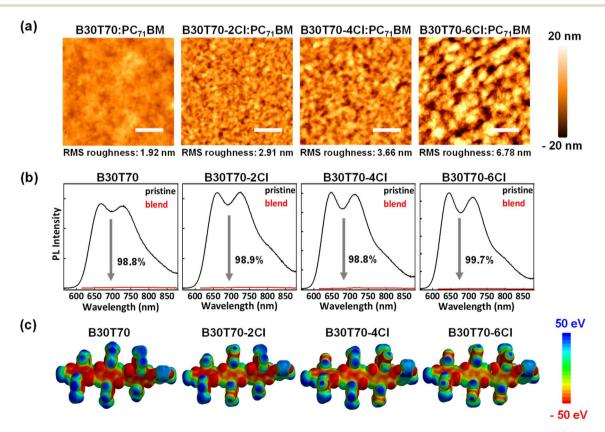
Fig. 4 (a) AFM surface topographic images of B30T70-XCl:PC<sub>71</sub>BM blends (the scale bar in the AFM images is 500 μm), (b) PL quenching efficiency of B30T70-XCl:PC<sub>71</sub>BM blend films, and (c) ESP map of B30T70-XCl units.
