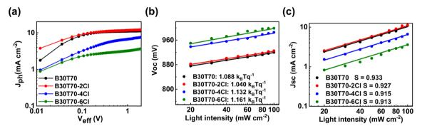
Fig. 6 (a)  $J_{\rm ph}-V_{\rm eff}$  curves under AM 1.5 G illumination. Light intensity dependence of (b)  $V_{\rm OC}$  and (c)  $J_{\rm SC}$ .
