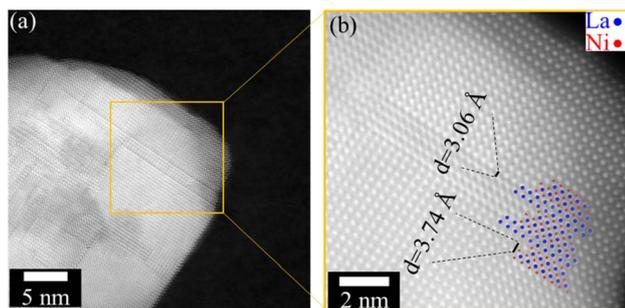
Fig. 3 (a) ADF image of  $\text{LaNiO}_3$ , showing the presence of multiple planar defects. (b) High-resolution HAADF-STEM micrograph. The positions of the La (blue) and Ni (red) columns are indicated.
