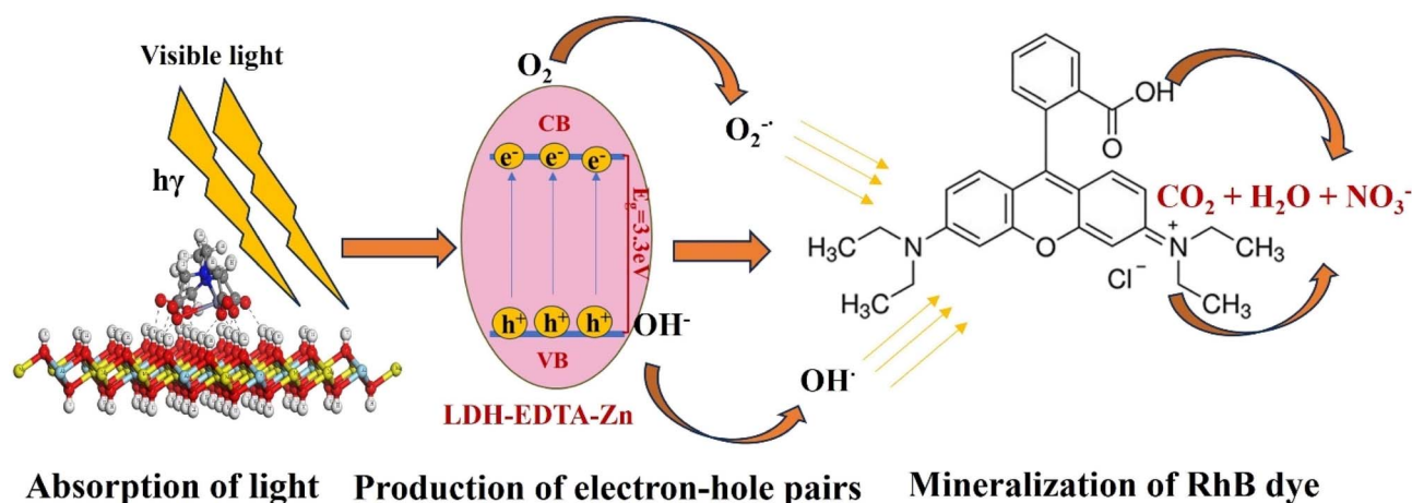
Fig. 13 A schematic representation of the photocatalytic degradation mechanism employed for RhB solution using the LDH-EDTA-Zn sample in the presence of an \text{H}_2\text{O}_2 initiator.
