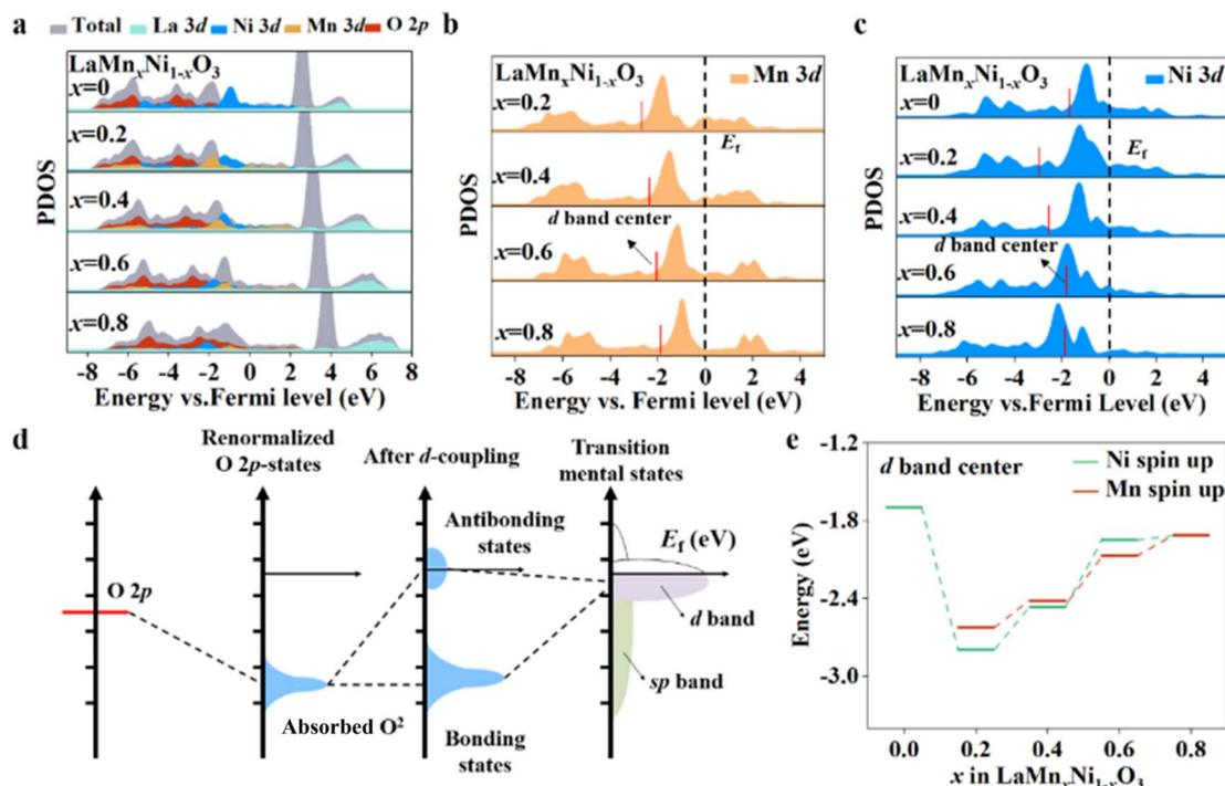
Fig. 6 (a) Comprehensive PDOS for various elements in  $\text{LaMn}_x\text{Ni}_{1-x}\text{O}_3$ . (b) PDOS of Mn 3d orbitals in  $\text{LaMn}_x\text{Ni}_{1-x}\text{O}_3$ . (c) PDOS of Ni 3d orbitals in  $\text{LaMn}_x\text{Ni}_{1-x}\text{O}_3$ . (d) Schematic diagram illustrating the shift of the d band center. (e) Trend analysis of the d band center variations for Mn and Ni.
