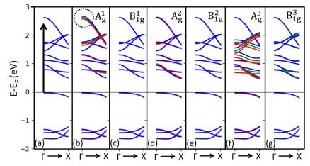
Fig. 7 Estimating the electron-phonon coupling using DFT calculations for the electronic dispersion of bulk PdSe<sub>2</sub> considering (a) unperturbed (green lines) and (b-g) different frozen phonons (blue and red for opposite displacements) (b)  $A_{q_r}^1$  (c)  $B_{1q_r}^2$  (d)  $A_{q_r}^2$  (e)  $B_{1q_r}^2$  (f)  $A_{q_r}^3$  and (g)  $B_{3q_r}^3$
