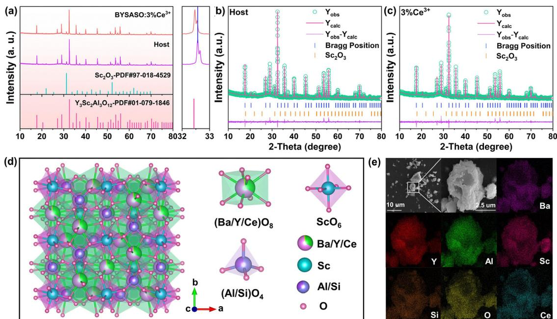
Fig. 1 (a) XRD patterns of the BYASO host and the as-prepared  $\text{BYASO}:3\%\text{Ce}^{3+}$  sample. The Rietveld refinements of the BYASO host (b) and the representative  $\text{BYASO}:3\%\text{Ce}^{3+}$  sample (c). (d) Crystal structure diagram of  $\text{BYASO}:3\%\text{Ce}^{3+}$  and the coordination environment of Ba, Y, Sc, Al, Si, O, Ce. (e) SEM patterns and elemental mapping of the optimal  $\text{BYASO}:3\%\text{Ce}^{3+}$  sample.
