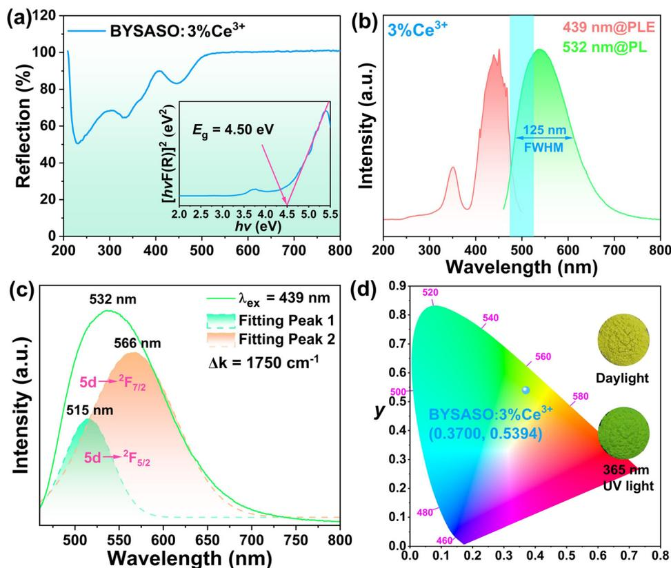
Fig. 2 (a) The DR spectrum and optical bandgap of BYASAO:3%Ce<sup>3+</sup>. (b) PLE and PL spectra of BYASAO:3%Ce<sup>3+</sup>. (c) Gaussian fitting curves of the PL spectrum for BYASAO:3%Ce<sup>3+</sup>. (d) CIE color coordinates of the BYASAO:3%Ce<sup>3+</sup> phosphor. The insets show the corresponding digital photographs under daylight and 365 nm near-UV lamp irradiation.
