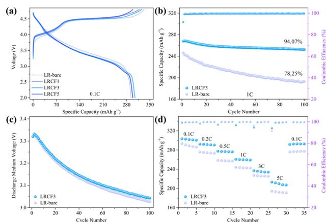
**Fig. 2** (a) Initial charge–discharge curves of LR-bare and LR-bare coated with different mass of CF. (b) Comparison of cycle performance and (c) voltage decay at 1C between LR-bare and LRCF3. (d) Rate performance of LR-bare and LRCF3.
