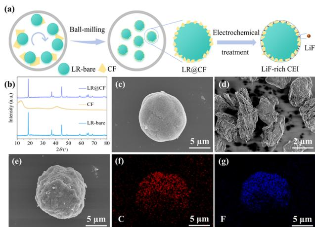
**Fig. 1** (a) Schematic diagram of the process of coating CF on LR-bare surface and the formation of LiF-rich CEI. (b) XRD patterns of LR-bare, CF and LR@CF. SEM images of (c) LR-bare, (d) CF and (e) LR@CF. The EDS mapping spectrum of (f) C and (g) F for LR@CF.
