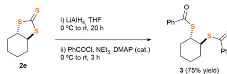
Scheme 2 Synthetic scheme for the derivatisation of TTC 2e into bis-thioester 3 .
