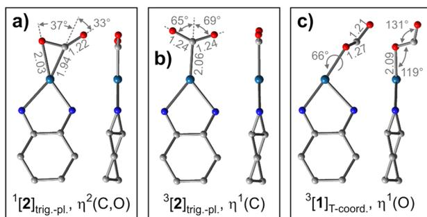
Fig. 8 DFT-optimized molecular structures of (carbon dioxide)[(1R,2R)-cyclohexanediamine]platinum(II) ([2]) in the singlet ground state (panel a) and the triplet states (panels b and c). In structure (a), the OCO bend angle is  $133^\circ$ . Level-of-theory: restricted ( $S = 0$ ) and unrestricted ( $S = 1$ ) B3LYP/GenECP. H-atoms hidden for clarity. All other atoms color-coded as follows: gray = C, blue = N, pale blue = Pt, red = O.
