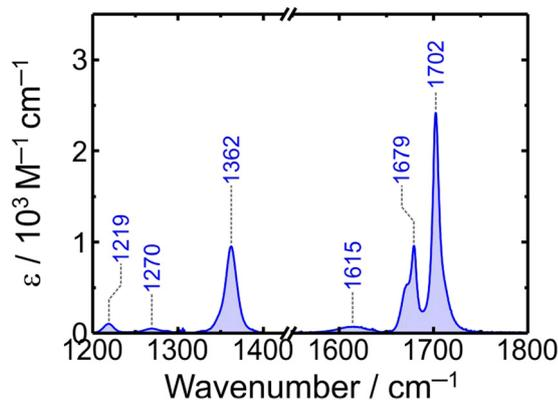
Fig. 2 Experimental FTIR-spectrum of [1] in DMSO (blue curve) at room temperature. The numbers indicate the peak positions in cm<sup>-1</sup>.
