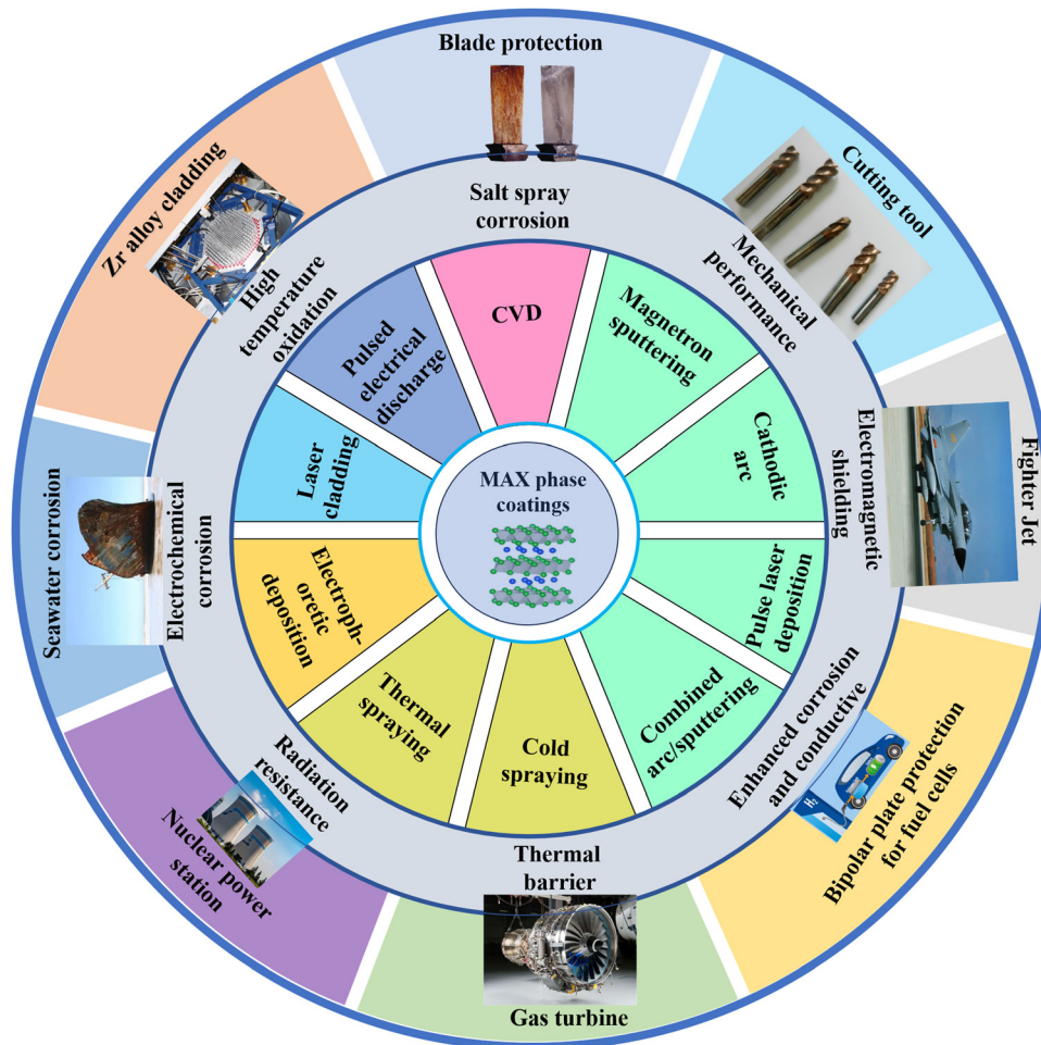
Fig. 4 Potential applications, properties and common preparation methods of MAX phase coatings.
