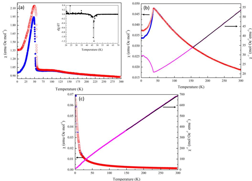
Fig. 6 Zero field cooled (blue) and field cooled (red) SQUID magnetometry data collected at 0.1 T and inverse ZFC susceptibility data where the black line shows the fit to the Curie–Weiss law for (a)  $\text{MnFeMo}_3\text{O}_8$  inset shows the  $d\chi/dT$  data highlighting  $T_N$  at  $\approx 46$  K, (b)  $\text{MnCoMo}_3\text{O}_8$  showing  $T_N \approx 35$  K and (c)  $\text{MnZnMo}_3\text{O}_8$  showing paramagnetic character.
