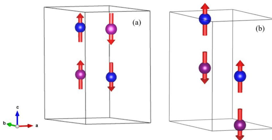
Fig. 7 Magnetic spin structure (red arrows) determined for (a)  $MnCoMo_3O_8$  and (b)  $MnFeMo_3O_8$  within the unit cell (black outline) at 2 K from the Rietveld refinement of powder neutron diffraction data. The blue and pink spheres represent manganese on the Mn1 (tetrahedral) and Mn2 (octahedral) crystallographic sites respectively.
