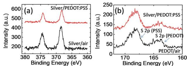
Fig. 6 XPS spectra of PEDOT:PSS layer and silver layer at different interface in (a) Ag 3d region and (b) S 2p region.
