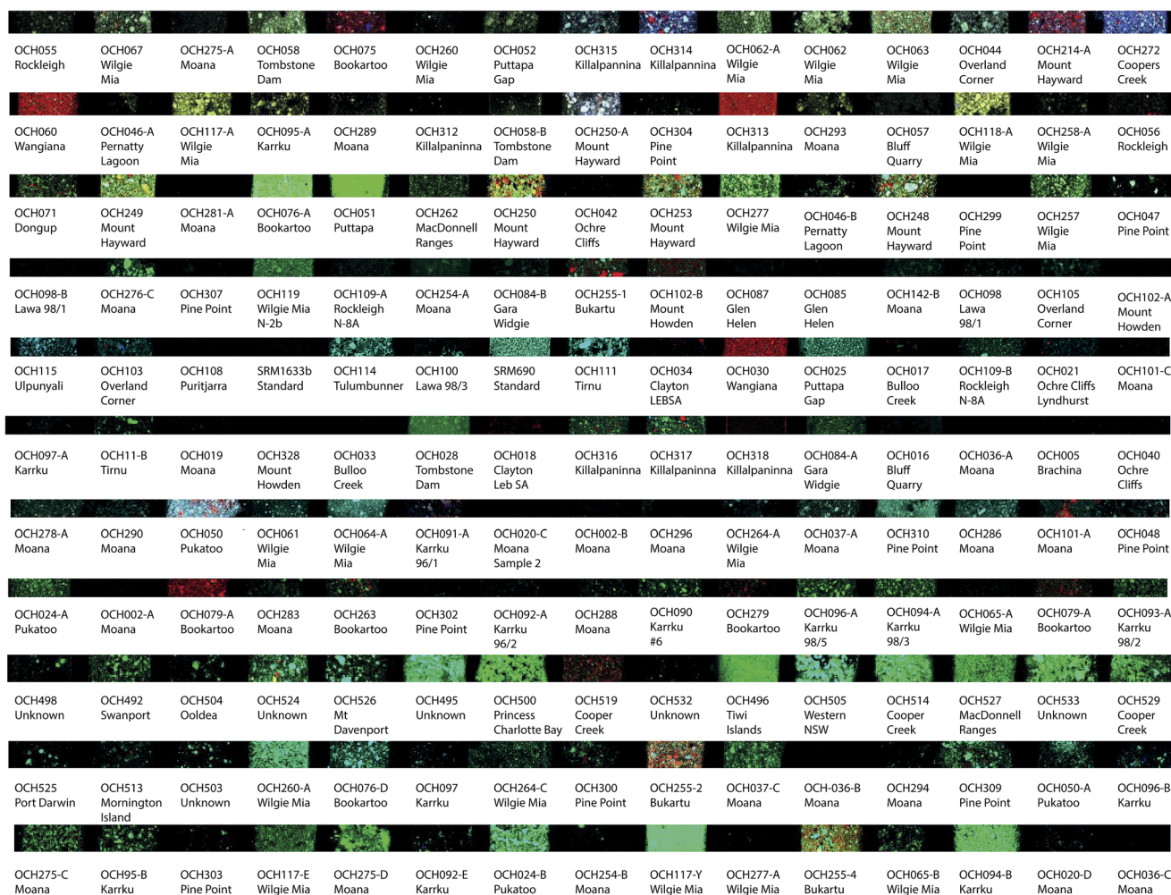
Fig. 7 Microelemental map of Ca, Fe and V for all 165 samples analysed in this study. Red indicates Ca, green indicates Fe and blue indicates V. Images are false coloured to demonstrate relative concentration intensities, with black the lowest and the indicated colour the highest.
