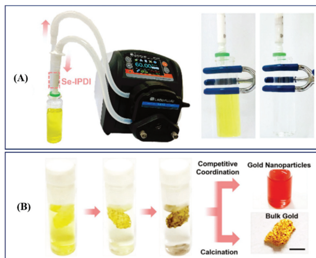
Fig. 11 (A) The equipment for simulating the dynamic extraction process in industrial treatment and the color change of the Au 3+ solution before and after treatment with the system; (B) procedure of gold extraction with Se-foam and posttreatments by competitive coordination or calcination. Reproduced with permission from ref. 216. Copyright 2020 WILEY-VCH Verlag GmbH & Co. KGaA, Weinheim.
