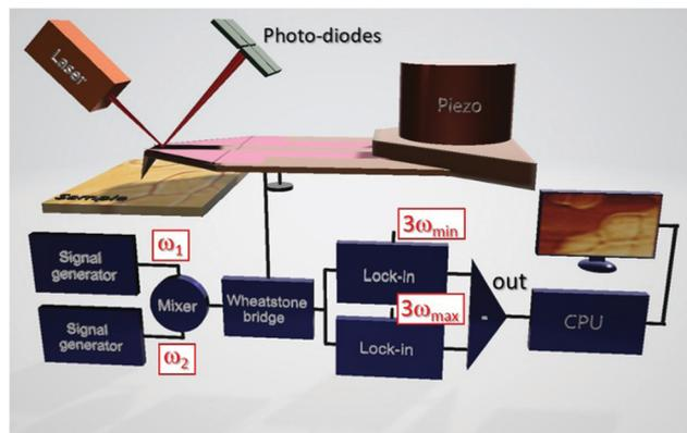
Fig. 6 Schematic illustration of extended quantitative thermal conductivity measurements by SThM applying the so-called  $3\omega$ -technique in the frequency domain. Reprinted with permission from ref. 50. Copyright (2019) American Chemical Society.
