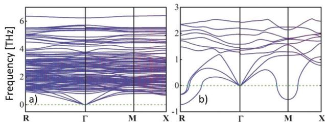
**Fig. 1** An ultralow thermal conductivity can be obtained from the calculated phonon dispersion curves in the low-frequency domain of (a) tetragonal MAPbI<sub>3</sub> at room temperature, while the thermal conductivity of (b) the cubic phase (> 54 °C<sup>33</sup>) is slightly larger, because the phonon group velocities are given by the gradient.<sup>31</sup> Copyright Wiley-VCH Verlag GmbH & Co. KGaA. Reproduced with permission.
