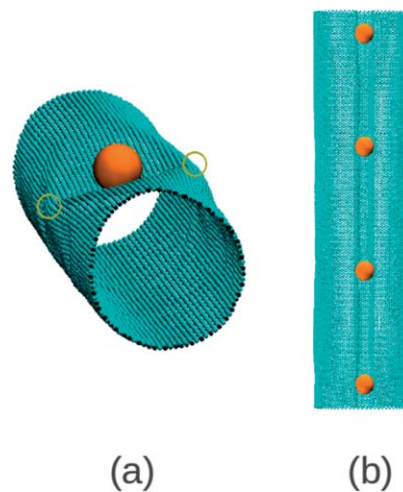
Fig. 4 (a) Transversal buckling caused by a large single point deformation. In this case l_p < L , and the side rings indicate the location of the transversal stress focus points. (b) Uniform axial buckling and nanotube radial collapse induced by four equidistant localized deformations such that 4l_p > L .
