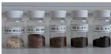
Fig. 1 Examples of the physical appearance of the pulp before and after pretreatment at 150 °C for 0.5 h, 1 h, 2 h and 4 h.
