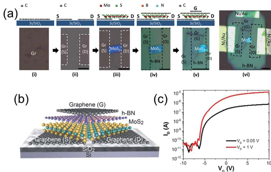
Fig. 5 (a) Schematics (not to scale) of the fabrication process steps (top) and the corresponding optical microscope images (bottom) of a representative graphene/h-BN/MoS<sub>2</sub> transistor. Scale bar is 5  $\mu\text{m}$  for all images. (b) and (c) Schematic illustration (b) and  $I_D$ - $V_G$  characteristics at different  $V_G$  (c) of the graphene/h-BN/MoS<sub>2</sub> transistor. Reprinted with permission from ref. 75. Copyright 2015 ACS.
