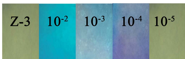
Fig. 5 Photographs of test strips (the concentration of Hg 2+ is 0 M, 10^{-1} M, 10^{-2} M, 10^{-3} M, 10^{-4} M, 10^{-5} M, both under an UV lamp at 365 nm).
