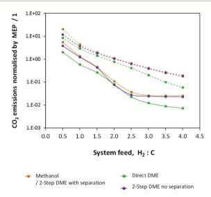
Fig. 12 CO<sub>2</sub> emissions normalised by the MEP for the methanol/DME production systems employing  $H_2$ -CO only (solid lines) and  $H_2$ -CO<sub>2</sub> only (dashed lines) feeds.
