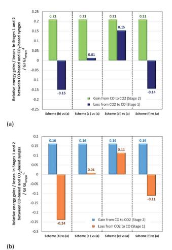
Fig. 14 Relative normalised energy losses in Stage 1 and gains in Stage 2 when (a) methanol and (b) direct DME systems are operated with CO-based and CO<sub>2</sub>-based syngas.
