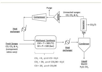
Fig. 2 A general process layout for a commercial methanol production system.
