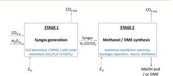
Fig. 1 Principal stages in methanol and DME syntheses from  $CO_2$  and  $H_2O$ . In Stage 1,  $CO_2$  and  $H_2O$  are converted to CO and  $H_2$  (syngas); in cases where  $CO_2$  it utilised directly only  $H_2$  is generated in Stage 1. In Stage 2, syngas is converted to methanol and/or DME.
