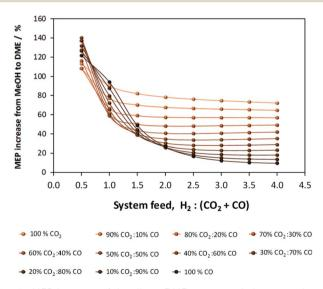
Fig. 6 MEP increase of the direct DME process relative to methanol alone; calculations based on reactor outputs at 250 °C and 50 bar in the absence of recycle.
