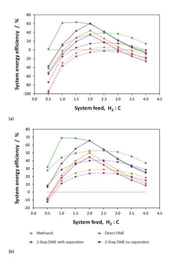
Fig. 9 Net energies obtained with (a) no energy savings and (b) maximum savings with the  $H_2$ -CO only (solid lines) and  $H_2$ -CO<sub>2</sub> only (dashed lines) system feeds for the four systems under investigation.
