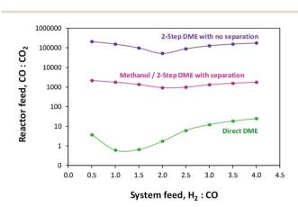
Fig. 11 CO :  $CO_2$  ratios in the recycle loops for the methanol/DME synthesis systems, fed only with H<sub>2</sub> and CO.
