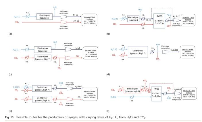
scheme (d), or performed in parallel with  $CO_2$  electrolysis as in scheme (e) if the  $H_2$ -CO ratio requires adjustment.
