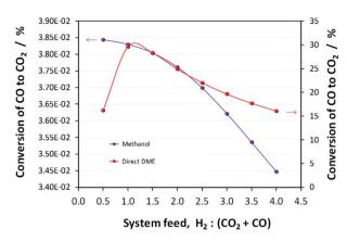
Fig. 7 Extents of CO conversion to  $CO_2$  via the water gas shift reaction during methanol and direct DME synthesis when a  $H_2$ -CO only feed was employed.
