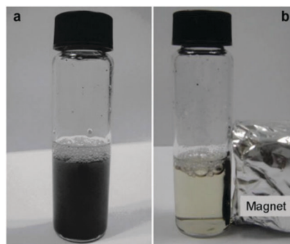
Fig. 37 Magnetic separation of a finely dispersed \text{Fe}_3\text{O}_4 based catalyst used for cellulose hydrolysis. Reproduced with permission from ref. 332. Copyright (2012) Springer Nature.
