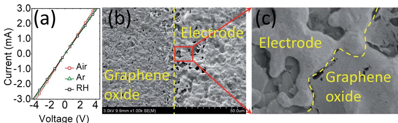
Fig. 2 Current–voltage ( $I$ – $V$ ) measurements performed in air, argon and 50% RH with a step size of  $\pm 0.01$  V (a). SEM micrograph showing the graphene oxide and electrode interface (b), and magnified view of the GO/electrode interface (c).
