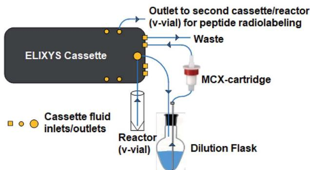
Fig. 3 Diagram of gross dilution set-up. Set-up allows [<sup>18</sup>F]FPy-TFP (5) purification via a 15 mL water dilution in an external flask, trapping on an Oasis MCX cartridge followed by a 5 mL water wash and 3 mL acetonitrile elution. All operations are fully automated via ELIXYS FLEX/CHEM® radiosynthesizer and no manual interventions required.
