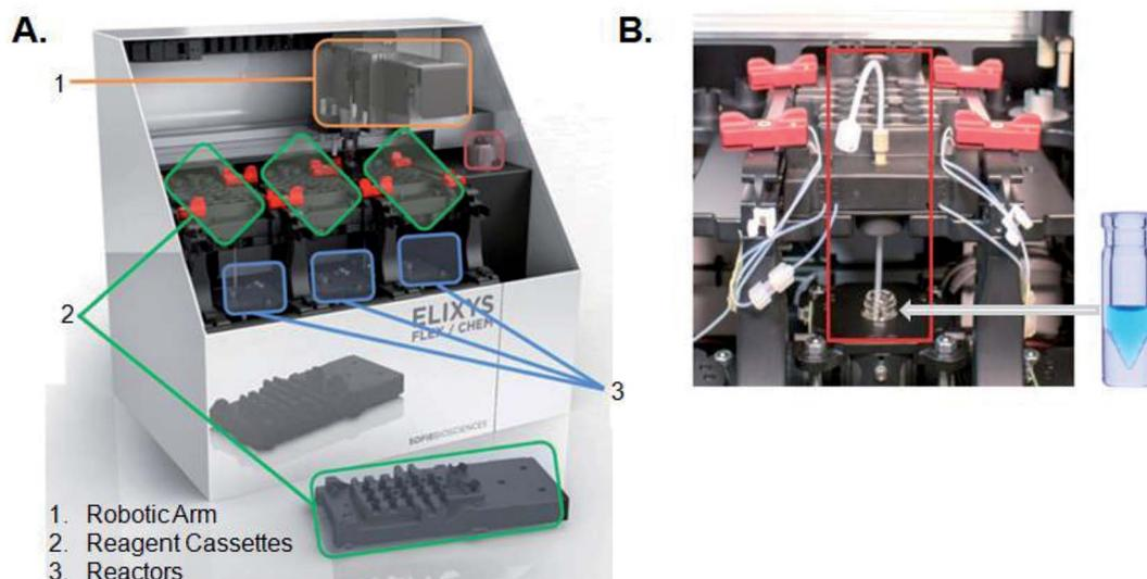
Fig. 2 (A) ELIXYS FLEX/CHEM® radiosynthesizer (B) zoom-in of a reagent cassette above one of the reactors containing the v-vial.
