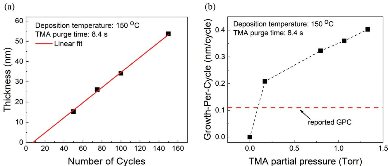
Fig. 2 (a) Measured film thickness vs. the number of cycles. The GPC is  $\sim 0.36$  nm per cycle with an x-intercept of 8 cycles. (b) Growth-per-cycle vs. the partial pressure of TMA. In these experiments, the partial pressure of EG was kept constant at 0.5 Torr and a timing sequence of (0.77, 8.4, 0.77, 2) was used. The GPC shows no signs of saturation and even at the lowest TMA partial pressure of 0.17 Torr, it is already higher than previously reported GPC.<sup>15</sup>
