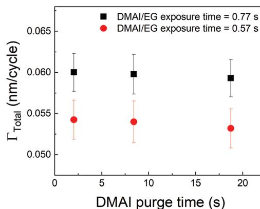
Fig. 9  $\Gamma_{\text{Total}}$  as a function of DMAI purge time. Unlike the observed decrease in  $\Gamma_{\text{Total}}$  with respect to TMA purge time, the DMAI purge time seems to have a negligible effect on  $\Gamma_{\text{Total}}$ .
