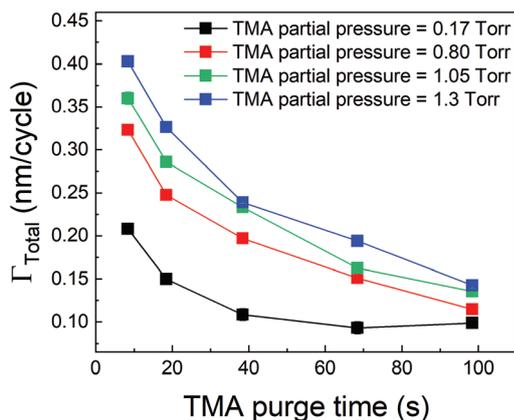
**Fig. 4**  $\Gamma_{\text{Total}}$  as a function of TMA purge time. In these experiments conducted at 150 °C, the EG dose, its purge time and TMA exposure time were kept constant while the TMA purge time was varied. For each TMA partial pressure,  $\Gamma_{\text{Total}}$  decreases with increasing TMA purge time and upon a long enough purge stabilizes at a steady-state value equal to  $\Gamma_{\text{MLD}}$ .
