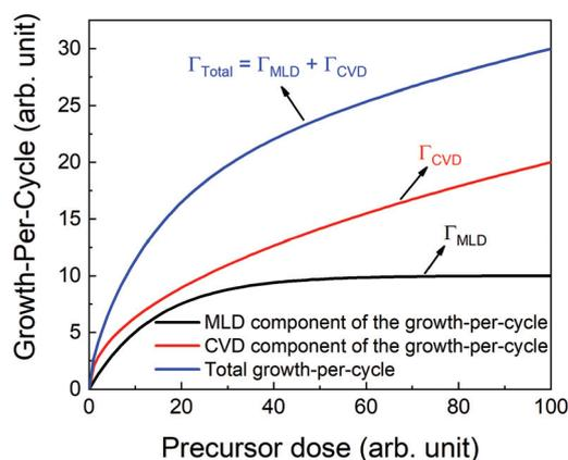
Fig. 3 A schematic showing different contributions in the total growth-per-cycle. The total GPC ( $\Gamma_{\text{Total}}$ ) could be seen as a result of contributions from the surface MLD reactions ( $\Gamma_{\text{MLD}}$ ) and the CVD reactions ( $\Gamma_{\text{CVD}}$ ).
