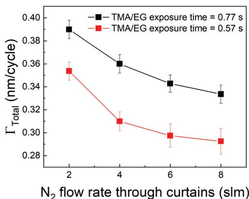
Fig. 8  $\Gamma_{\text{Total}}$  as a function of  $\text{N}_2$  flow through the gas curtains. In these experiments, the partial pressures and exposure times of both TMA and EG were kept constant while only the  $\text{N}_2$  flow through the four curtains was varied from 2 to 8 slm (0.5 to 4 slm per curtain).
