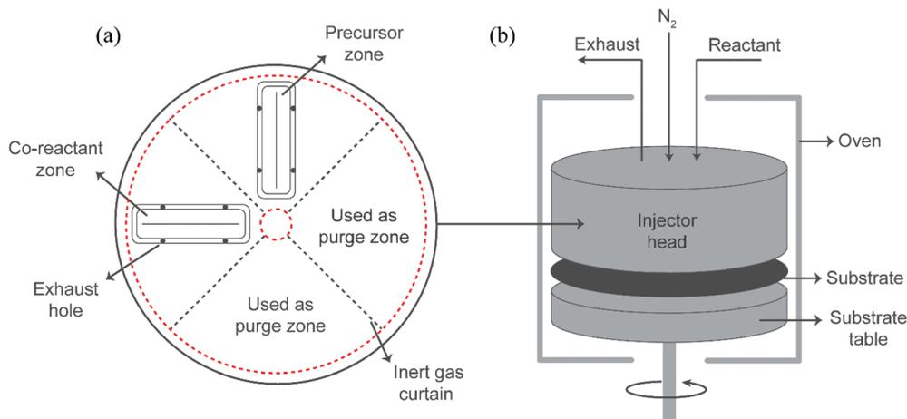
**Fig. 1** (a) A schematic drawing of the bottom-side of the Spatial ALD injector head. (b) A schematic drawing of the entire reactor. The substrate is placed in between the stationary injector head and the rotary substrate table. Each rotation of the substrate table sequentially exposes the substrate to the precursor and the co-reactant and corresponds to one MLD cycle. The entire setup is placed inside an oven heated to the desired deposition temperature.
