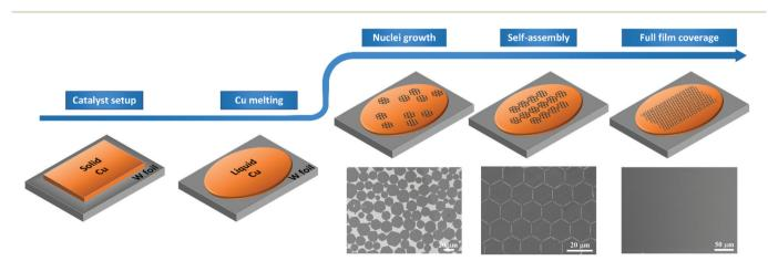
Fig. 1 Schematic illustration of the CVD growth process of graphene on liquid Cu. SEM images are indicative of dispersed graphene hexagonal flakes, self-ordered graphene hexagonal flakes and continuous uniform graphene film, respectively (this figure has been adapted/reproduced from ref. 42 with permission from PNAS, copyright 2012).
