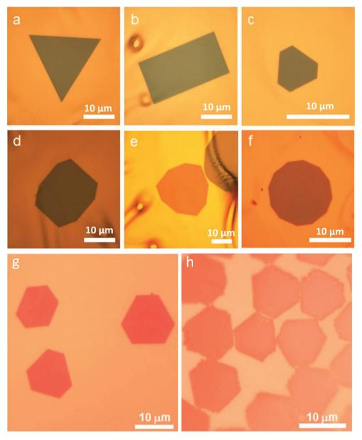
Fig. 10 Optical images of 2D  $\alpha$ -Mo<sub>2</sub>C crystals with various shapes. (a) Triangle, (b) rectangle, (c) hexagon, (d) octagon, (e) nonagon, and (f) dodecagon. All the scale bars are 10 μm. Optical images of 2D (g) WC crystals, (h) TaC crystals. Reprinted with permission from Springer Nature, Nature Materials<sup>148</sup> (large-area high-quality 2D ultrathin Mo<sub>2</sub>C superconducting crystals, C. Xu et al., 2015).
