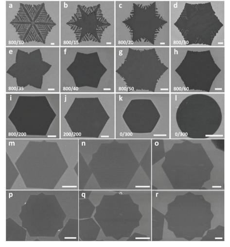
Fig. 5 SEM images of GFs grown on a liquid Cu surface with different shapes formed by varying the Ar: H<sub>2</sub> ratio (a-1). Reprinted with permission from Springer Nature, NPG Asia Materials<sup>74</sup> (self-organized graphene crystal patterns, B. Wu et al., 2013). Formation of tips in hexagonal graphene grains by incremental additions to the CH<sub>4</sub> flow (m-r). Reprinted with permission from ref. 75. Copyright 2014 Wiley-VCHd. All scale bars are 5 µm.
