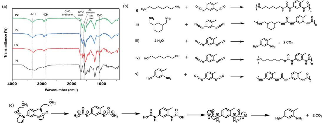
**Fig. 2** (a) FT-IR spectra of the polyurea (P2–3) and polyurethane/urea (P6–7) nanocapsules. (b) Scheme for the reactions between the diamines monomers and from hydrolyzed diisocyanates, water, and diols with the toluene-2,4-diisocyanate (TDI) (c) Mechanism of the hydrolysis of isocyanate and decarboxylation of the carbamic acid in the presence of water.
