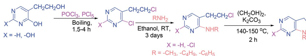
Scheme 19 Synthesis of 5,6-dihydropyrrolo[2,3- d ]pyrimidines.
