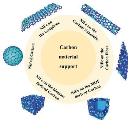
Fig. 9 NiFe alloys supported on different conductive substrates.
