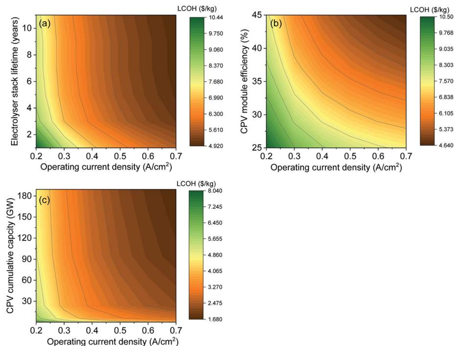
Fig. 5 Contour plots showing the sensitivity of  $H_2$  cost to: (a) electrolyser stack lifetime, (b) CPV module efficiency and (c) CPV cumulative installed capacity versus operating current density of the electrolyser.
