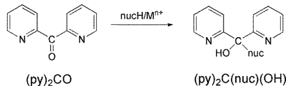
Scheme 1 General reactivity pattern of coordinated di-2-pyridyl ketone, (py) 2 CO. The neutral nucleophile is represented by nucH and can be H 2 O, alcohols, Me 2 CO, MeCN, pyrazoles, secondary amino acids, etc. The attack of the nucleophile on the carbonyl carbon atom requires its deprotonation, which is often achieved by an external base. M n+ is the metal ion ( n = 2, 3 ). When nucH is H 2 O, the product is the gem -diol derivative of (py) 2 CO, (py) 2 C(OH) 2 , whereas the addition of alcohols (ROH) produces the hemiacetal form of (py) 2 CO, (py) 2 C(OR)(OH). Note that compounds (py) 2 C(nuc)(OH) and their anionic forms do not exist as free species, but only in the presence of metal ions ( i.e. as ligands in their respective metal complexes). Important note: in the abbreviations of the ligands, the carbonyl oxygen atom is written without parenthesis, whereas the oxygen atoms which form single bonds with the central carbon are written within parenthesis.
