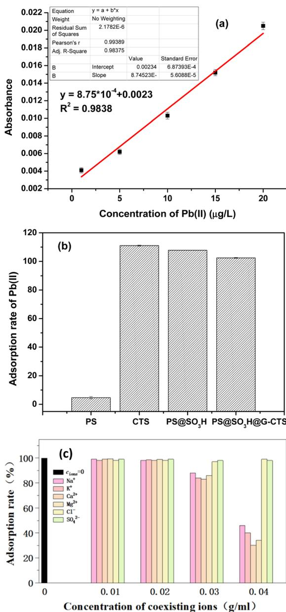
Fig. 8 Adsorbability comparisons for Pb(II) ((a) the standard curve of Pb(II); (b) the adsorption rates of Pb(II) by PS, CTS, PS@SO<sub>3</sub>H and PS@SO<sub>3</sub>H@G-CTS; (c) anti-interference).
