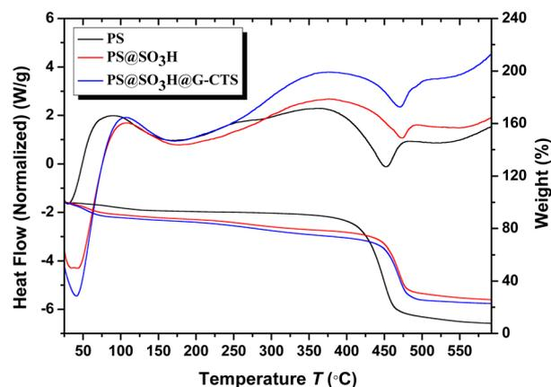
Fig. 6 TGA and DSC of PS, PS@SO<sub>3</sub>H and PS@SO<sub>3</sub>H@G-CTS.
