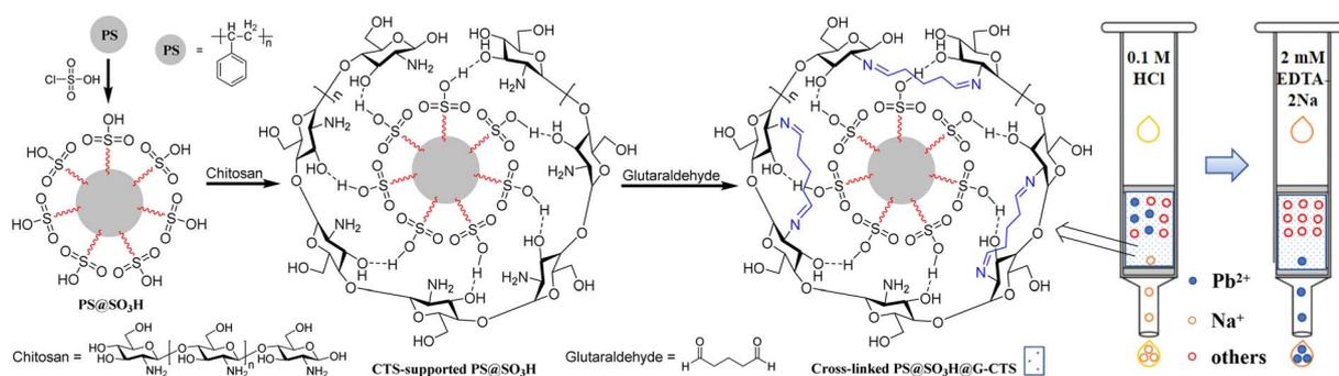
Scheme 1 Synthetic routes of polystyrene–chitosan composite microspheres.
