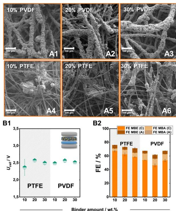
Fig. 4 Scanning electron microscopy (SEM) investigation of PVDF (A1–A3) and PTFE bound electrodes (A4–A6). Effect of the binder nature and content on the ECH of MBY at 80 mA cm<sup>-2</sup>. The obtained cell voltage (B1) and faradaic efficiency (B2). Here, FE<sub>MBX</sub> (C) and FE<sub>MBX</sub> (A) (X: E, A) correspond to the FE values of ECH products detected in the catholyte and anolyte after electrolysis, respectively.
