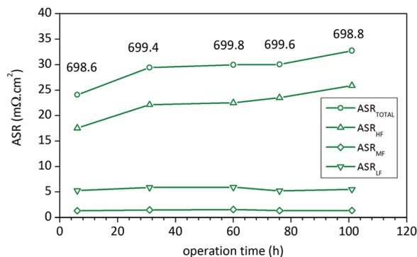
Fig. 7 Long-term operation test of LSC75–GD<sub>MW</sub>25 cathode at 700 °C during 101 h under synthetic air flow. The evolution of each component with time shows the origin of the increment in  $ASR_{TOTAL}$  observed during the first hours of operation. The inserted numbers indicate the temperature of the sample in °C when the measurement was performed.
