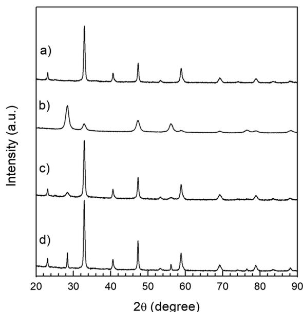
Fig. 3 XRD patterns. (a) LSC nanopowders; (b) GDC powder with particles of spherical shape; (c) LSC75–GD<sub>MW</sub>25 cathode before the sintering process; (d) LSC75–GD<sub>MW</sub>25 cathode after 2H at 850 °C.
