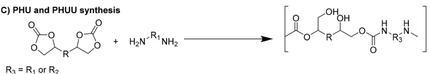
Fig. 11 Polyhydroxiuethane (PHU) and PHUU synthetic route.
