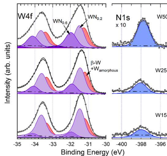
Fig. 6 W4f and N1s spectra for W thin film growth in reactive gas mixtures with N<sub>2</sub> (%): 15, 25, and 50. With the progressive incorporation of nitrogen, we identified different tungsten nitride phases:  $\sim$ WN<sub>0.2</sub> and  $\sim$ WN<sub>0.6</sub>.
