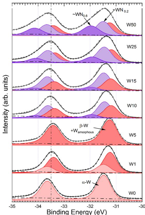
Fig. 5 W4f spectra for W thin film growth in reactive gas mixtures with N<sub>2</sub> (%): 0, 1, 5, 10, 15, 25, and 50. With the progressive enhancement of N<sub>2</sub>, we identified different W-based phases:  $\alpha$ -W,  $\beta$ -W, amorphous W, WN<sub>0.2</sub>, and WN<sub>0.6</sub>.
