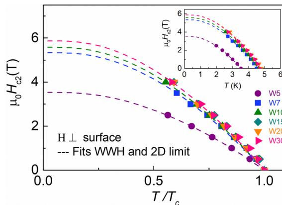
**Fig. 4** Upper critical field as a function of the reduced temperature ( $T/T_c$ ) for 20 nm thick W thin film growth using different concentrations of N<sub>2</sub> in the gas mixture. Inset: Similar to the main panel but with absolute temperature in the  $x$ -axis. Dashed lines correspond to the fit using the WHH model for dirty superconductors.
