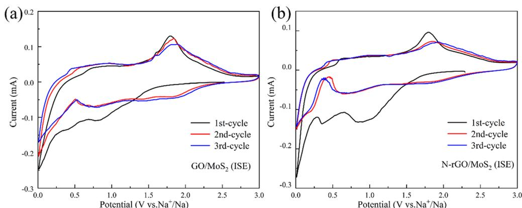
Fig. 5 CV curves at a scanning rate of  $0.2 \text{ mV s}^{-1}$  of (a) GO/MoS<sub>2</sub> (ISE) and (b) N-rGO/MoS<sub>2</sub> (ISE).
