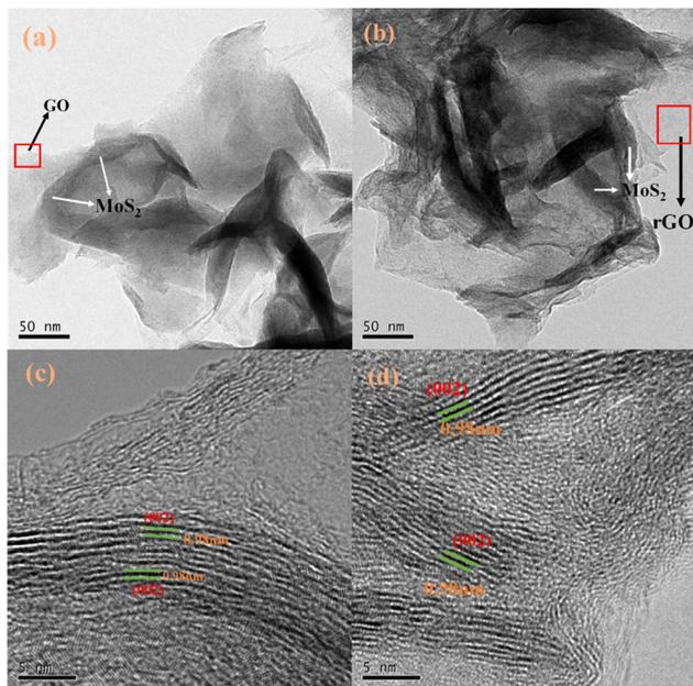
Fig. 3 TEM images of (a) GO/MoS<sub>2</sub> (ISE) and (b) N-rGO/MoS<sub>2</sub> (ISE). HRTEM images of (c) GO/MoS<sub>2</sub> (ISE) and (d) N-rGO/MoS<sub>2</sub> (ISE).
