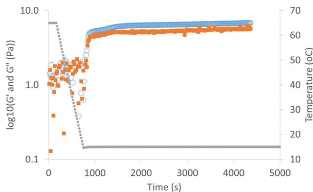
**Fig. 2** Plot of  $G'$  (open blue circles) and  $G''$  (closed red squares) against temperature (closed grey circles) and time for AMF sample provided by Arla foods, measured in an Anton Paar MCR302 oscillatory rheometer at a controlled strain of 0.001% and a frequency of 1 Hz. Plate inner diameter 50 mm, cone: 23 mm, angle 1°, shear rate 1 s<sup>-1</sup>.
