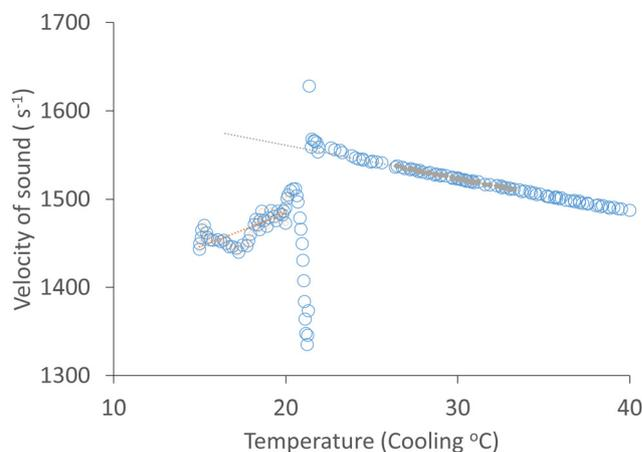
**Fig. 3** Velocity of sound in AMF, measured in the Resoscan and cooled from 40 °C to 15 °C over 12 hours. Fit to cooling data between 40 °C and 26 °C,  $y = -3.7629x + 1636.2$ ,  $r^2 = 0.992$ ; fit to cooling data between 20 °C and 15 °C,  $y = 7.5535x + 1332.7$ ,  $r^2 = 0.5848$ .
