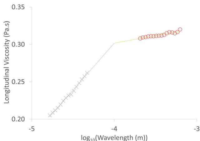
Fig. 5 Longitudinal viscosity plotted against wavelength at 40 °C, derived from ultrasound attenuation data such as that shown in Fig. 4. Short wavelength – black crosses, power law fit  $y = 2.4562x^{0.2427}$ ,  $r^2 = 0.996$ . Long wavelength – red open circles, power law fit,  $y = 0.4125x^{0.0349}$ ,  $r^2 = 0.938$ .
