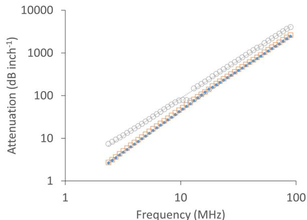
Fig. 4 Selected attenuation spectra for anhydrous milk fat. Filled blue circles, 43 °C; red open squares, 40 °C; black open circles, 23 °C. 43 °C fit,  $y = 0.56x^{1.885}$ ,  $r^2 = 0.9992$ . 23 °C fit,  $y = 1.464x^{1.7703}$ ,  $r^2 = 0.9976$ .
