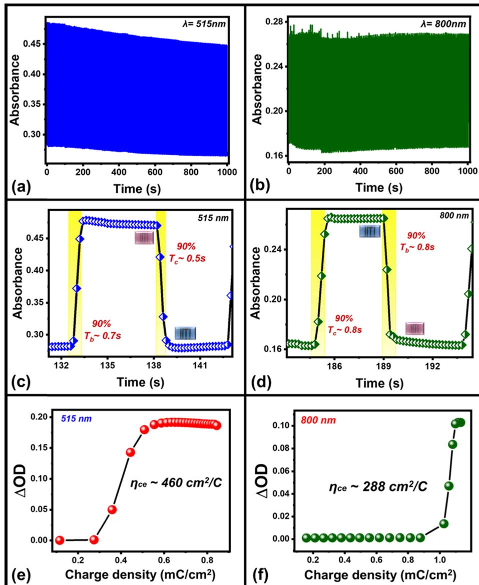
Fig. 4 (a) *In situ* bias-dependent multiple switching cycles of the device between ON and OFF states in the voltage window ( $\pm 1.5$  V) in the visible and infrared (IR) wavelength region in (b) and (c) single switching cycle at 515 nm wavelength, (d) response time of the device in the same fixed voltage window at 800 nm wavelength, and the corresponding estimated coloration efficiencies of the device in (e) and (f).
