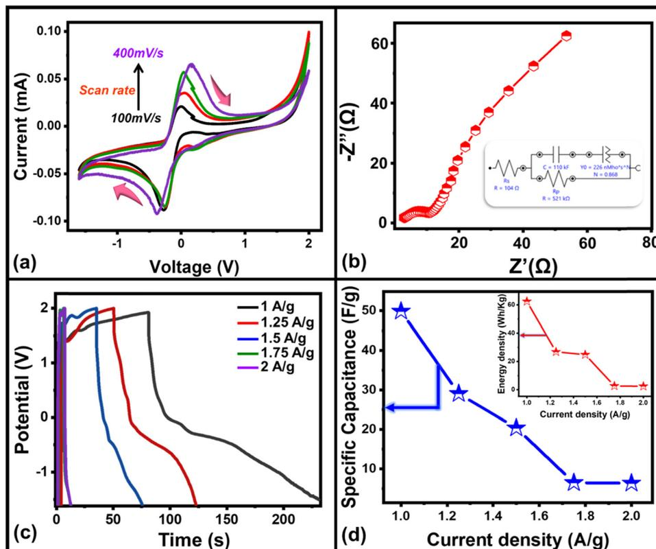
Fig. 5 (a) Cyclic voltammetry of the device for different scan rates, (b) Nyquist plot (inset: equivalent electric circuit), (c) charging/discharging curves with increasing current densities and (d) varying specific capacitance value along with the energy density variation of the device in the inset.
