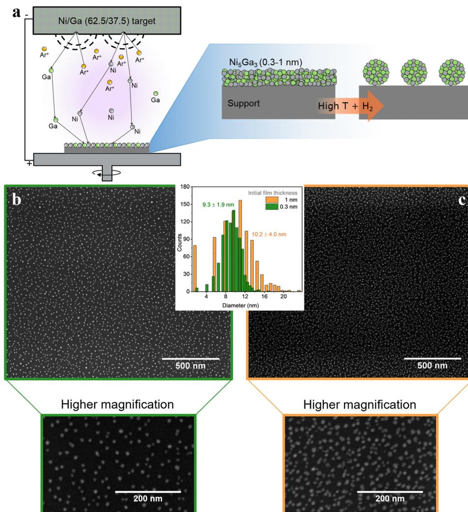
Fig. 8 (a) Nanoparticle synthesis schematics, combining magnetron sputtering and annealing; (b) and (c)  $\text{Ni}_5\text{Ga}_3$  thin films of 0.3 (green) and 1 nm (orange), respectively, on an  $\text{SiO}_2$  (50 nm)/Si (350  $\mu\text{m}$ ) support annealed at  $750^\circ\text{C}$  for 30 min in 10%  $\text{H}_2$  in He. SEM images were acquired at 5 kV and 0.1 nA.
