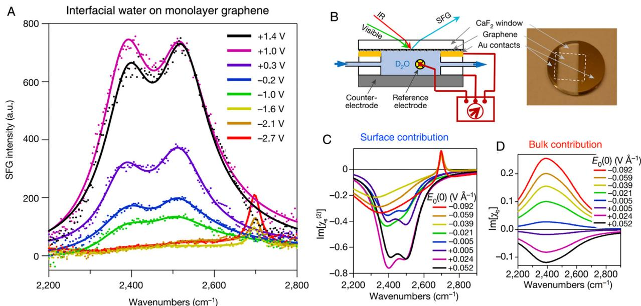
**Fig. 10** (A) *In situ* SFG spectra of D<sub>2</sub>O at the graphene electrode (no electrolyte is added to D<sub>2</sub>O). The potential is referenced to a Ag/AgCl electrode. (B) Schematic of an electrochemical cell and the corresponding photograph of a graphene electrode for SFG experiments. (C) and (D) The extracted surface (C) and bulk (D) contribution from SFG spectra as a function of the applied field. Reproduced with permission from ref. 140. Copyright 2021 Springer Nature.
