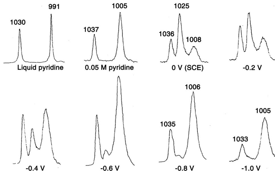
Fig. 5 First SERS experiment by Fleischmann *et al.* in 1974, in which the adsorption of pyridine was studied on a roughened Ag electrode surface. Reproduced with permission from ref. 15. Copyright 1974 Elsevier B.V.
