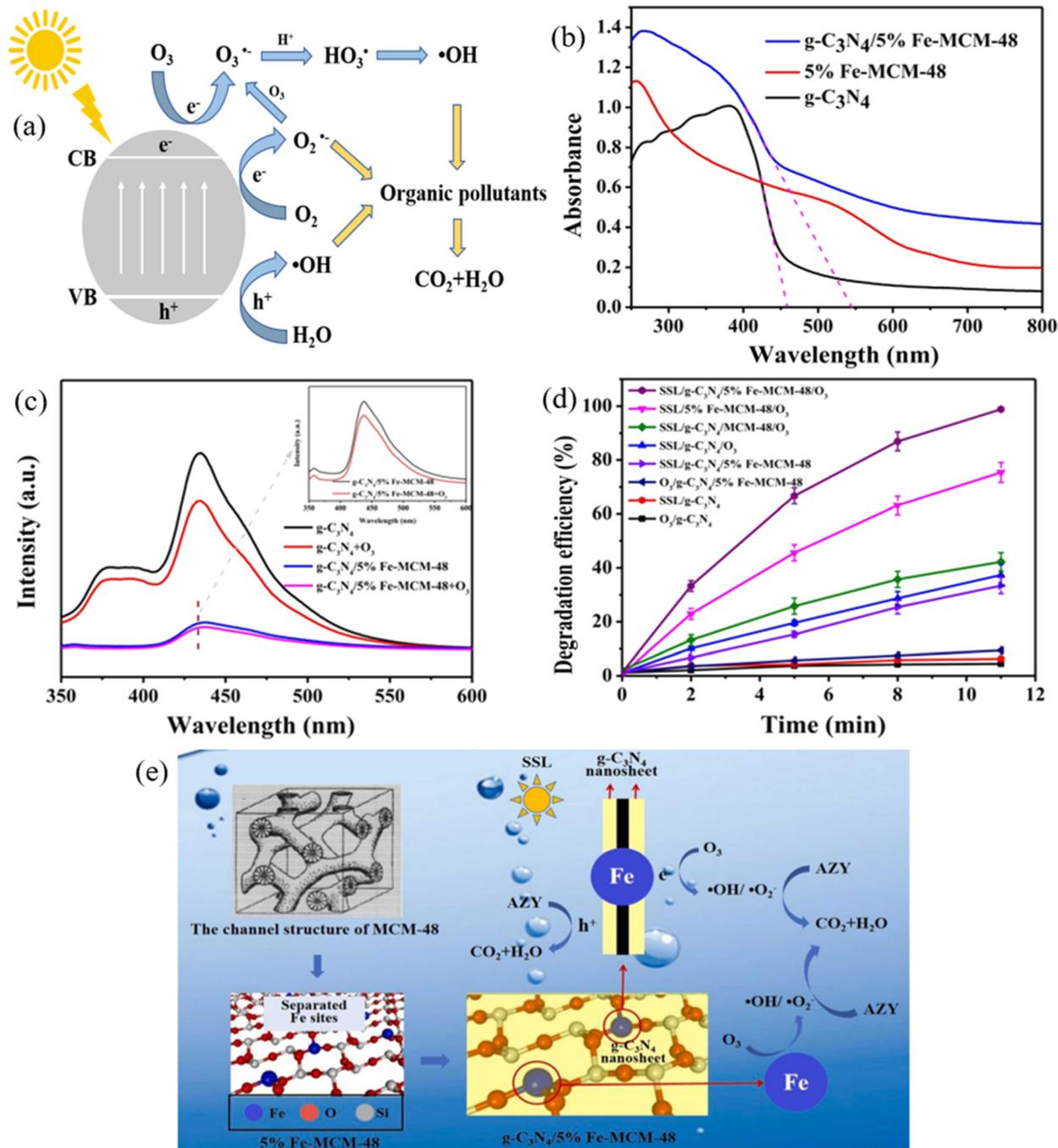
Fig. 7 (a) Schematic diagram showing the mechanisms of photocatalytic ozonation using MRNPCs; (b)  $N_2$  adsorption-desorption isotherms, (c) light adsorption ability, and (d) PL spectra of  $g-C_3N_4$ , 5% Fe-MCM-48, and  $g-C_3N_4/5\% Fe-MCM-48$ ; (e) proposed mechanisms of azithromycin degradation by photocatalytic ozonation using  $g-C_3N_4/5\% Fe-MCM-48$ . Reproduced from ref. 170 with permission from Elsevier, copyright 2023.
