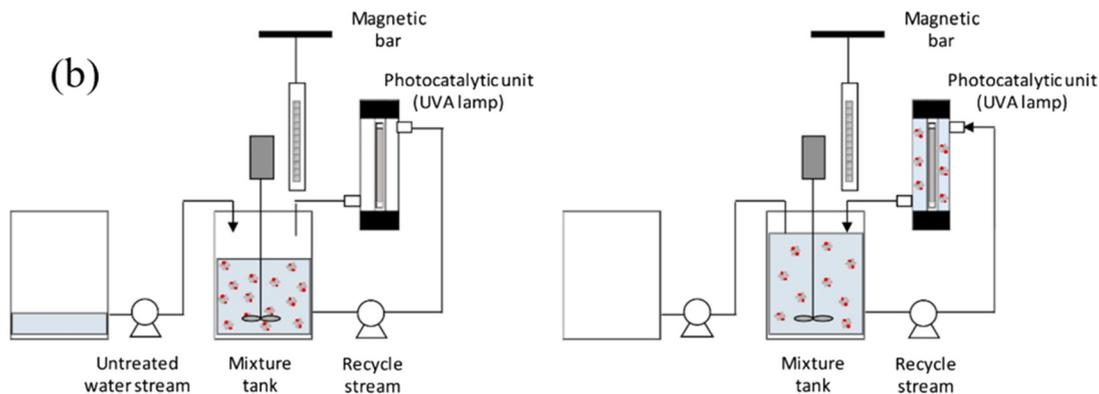
**Fig. 8** (a) Challenges of MRNPCs in practical applications; (b) operation of magnetic photocatalytic reactor: 1) loading of MRNPCs and water, 2) continuous phototreatment; 3) end of phototreatment, 4) MRNPCs recycling. Reproduced from ref. 70 with permission from Elsevier, copyright 2019.
