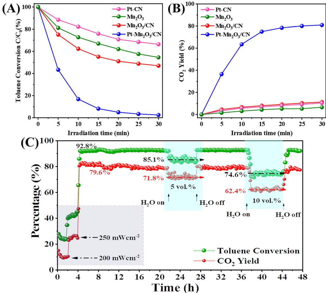
Fig. 3 Photothermal catalytic oxidation of toluene, (A) toluene conversion, and (B) CO<sub>2</sub> yield during the static reaction with 400 ppm toluene over the different catalysts, (C) toluene conversion and CO<sub>2</sub> yield during the continuous flow reaction over the Pt-Mn<sub>2</sub>O<sub>3</sub>/CN catalysts (full solar spectrum irradiation with 300 mW cm<sup>-2</sup> light intensity, 200 ppm toluene, and WHSV = 30 000 mL g<sup>-1</sup> h<sup>-1</sup>).
