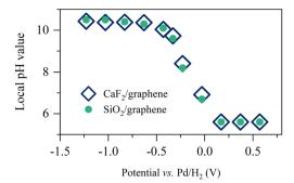
Fig. 2 Pseudocapacitive pH changes near the graphene electrode. Inferred local pH value as a function of the applied potentials for the  $SiO_2$ - and  $CaF_2$ -supported graphene electrodes. The data for the  $CaF_2$ -supported graphene electrode is adapted from ref. 10.
