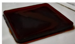
Fig. 12 Image of the obtained ionogel.
